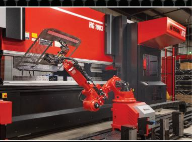
The HG 1003 ARs is designed to handle sheets up to 39" x 31" and the system's robot can support loads up to 44 lbs.
