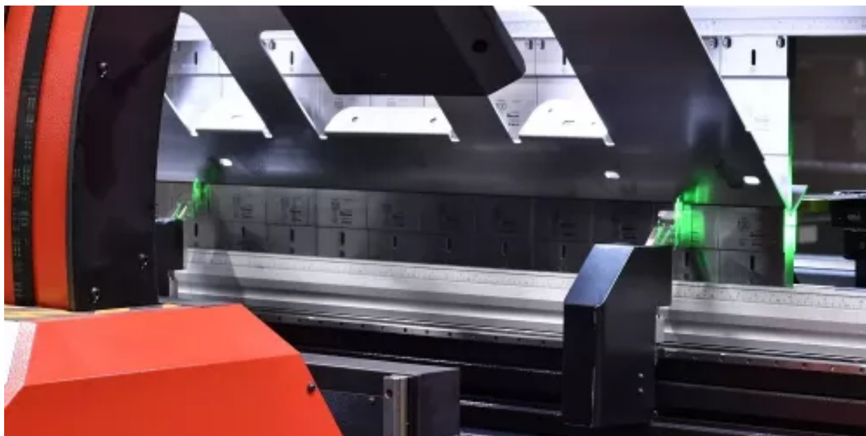
A sheet follower helps an operator form an edge flange on a complicated part, using one of the company’s two ATC press brakes. Bend indicators use probes to measure the angle in-process.
