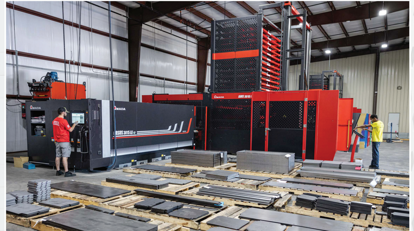
Keith Dunham (left) stands in front of the company's latest investment in flexible automation—a TK 3015L automated part sorting cell. The system automatically sorts and stacks parts according to their next production phase, reducing downstream labor and errors. Upstream, the TK is fed by an ORSUS 3015 Aje fiber laser and an AMS 3015 CLT automated tower material handling and storage system (above).
