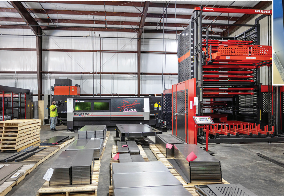
Located next to the new TK 3015L, the ENSIS 3015 AJ is paired with an AMS 3015 CLT multi-shelf automated material handling/storage tower, enabling 24/7 processing of parts for a wide variety of custom-designed secure storage solutions.
