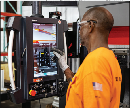
Offline programming with 3D bend simulation and an intuitive touch-screen control ensures precise, repeatable bending results across operators with varying skill levels.
