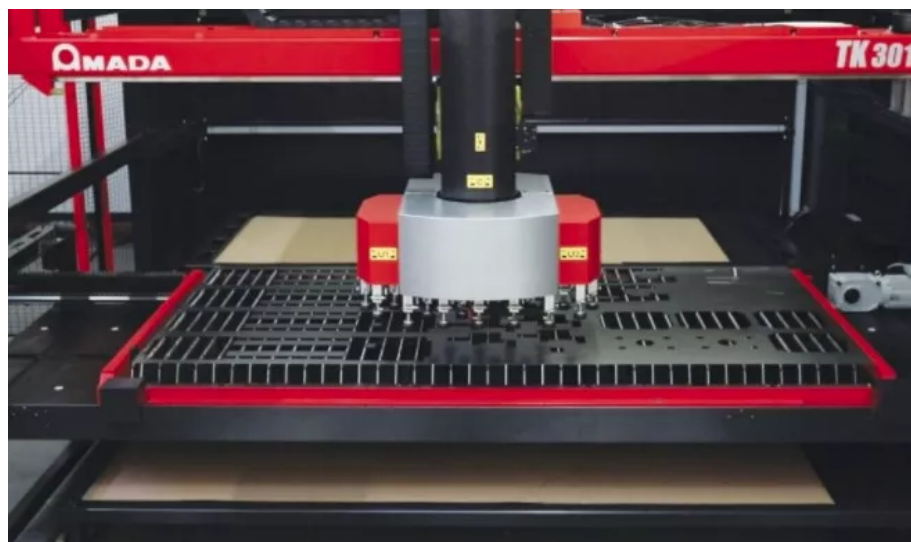
Figure 3 With the right nesting and programming strategy, part removal systems should be able to lift parts cleanly out of the nest.
