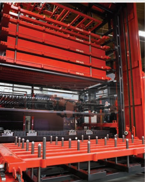
ASLUL300 Load/unload system — Automation is essential to maximize machine potential and achieve lights-out production.
