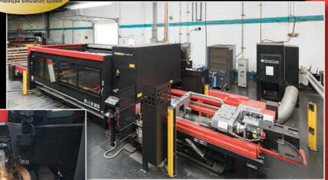
The Rotary Index on the FOM2 RI is located on one of three shuttle pallets — making it extremely easy and fast to switch from flat sheet cutting to tube or pipe cutting.
