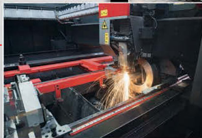
The Rotary Index on the FOM2 RI is located on one of three shuttle pallets — making it extremely easy and fast to switch from flat sheet cutting to tube or pipe cutting.
