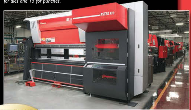
The Automatic Tool Changer (ATC) is equipped with 18 magazines for dies and 15 for punches.
