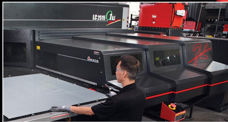
The LC 2515 CI AJ combines the force of a 22-ton turret punch press with the flexibility of a 2kW fiber laser. A 49-station MPT (Multi-Purpose Turret) provides for unique forming and tapping features — further enhancing productivity and reducing secondary operations.
