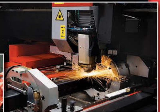
The FOM2 RI’s Rotary Index is located on one of three shuttle pallets — making it extremely easy to switch from flat sheet cutting to tube or pipe cutting.
