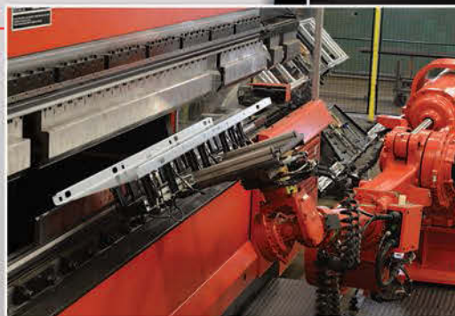
The Astro 165W Robotic Bending System provides the ideal high-speed solution for large parts and thick materials.
