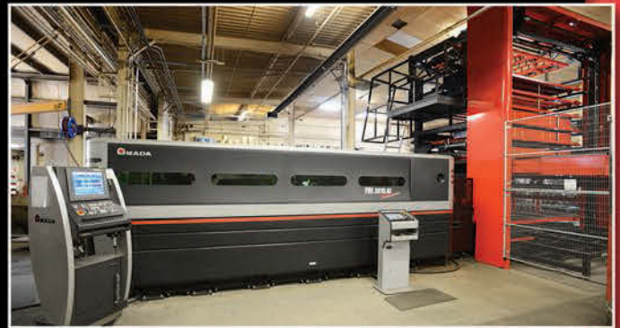
The FOL 3015 AJ Fiber Laser achieves cutting speeds up to 9,400 inches per minute and rapid traverse of over 13,000 inches per minute. ASLUL automation provides high-speed material handling at a rate to match the productivity of the Fiber Laser.
