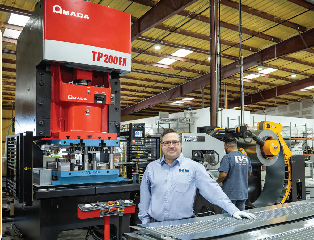
Forming: TP 200 FX 220-Ton Single Crank Stamping Press with a Coil Straightener-Feeder
