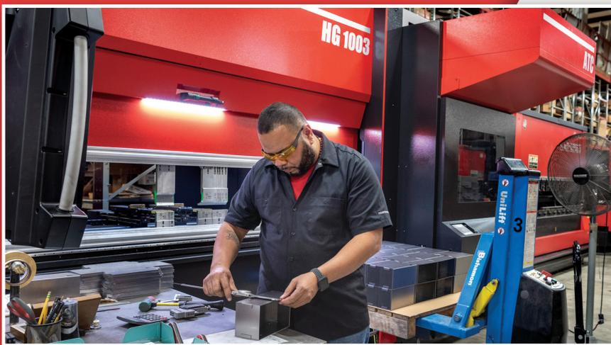
(Above: HG 1003 ATC) Complex bending is greatly simplified by the AMNC 3i control. The control and the Automatic Tool Changer (ATC) work together to make certain all tools can be staged at the same time. As a result, Vernier's operators can run more jobs in a single setup to optimize throughput.
