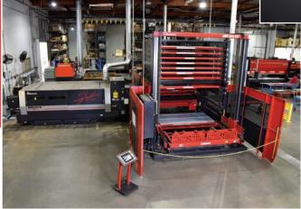
A ten-shelf, Automated Tower System provides for nonstop productivity — keeping pace with unique thin-to-thick cutting capabilities and high-speed processing of the ENSIS 3015 Fiber Laser.
