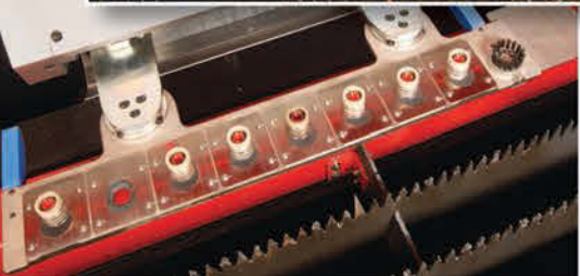
An 8-station changer automatically changes, cleans and calibrates the nozzle based on material processing requirements
