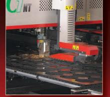
Mounted on the CI's frame, an automated part removal system places parts on a conveyor with multiple feed and stacking options — reducing labor and handling costs while taking productivity to a higher level.
