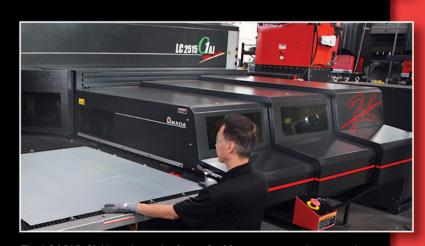
The LC 2515 C1 AJ combines the force of a 22-ton turret punch press with the flexibility of a 2kW fiber laser. A 49-station MPT (Multi-Purpose Turret) provides for unique forming and tapping features — further enhancing productivity and reducing secondary operations.
