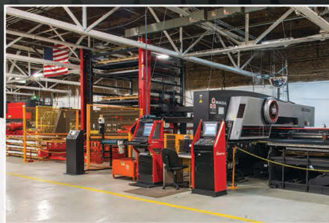
EMLK 3610 NT punch/laser combination machine (with advanced automation).
